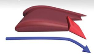
Plain flaps lower the wing's trailing edge increasing its curvature and, therefore, its lift.
