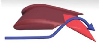
Fowler flaps move rearward and downward increasing the wing area and curvature.
